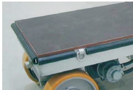
A rubber guard around the trolley prevents the arising of sparks.
