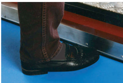
A safety guard around the Mover minimises injuries and prevents debris from entering the air bearing area.
